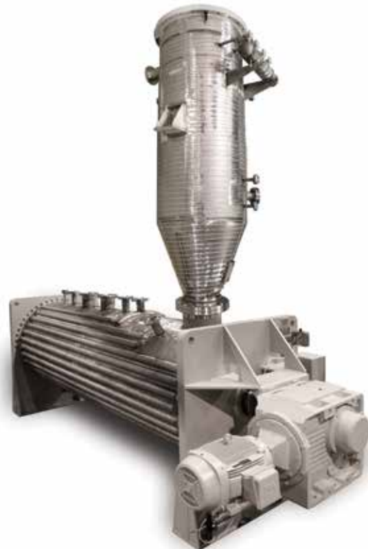
200 ft³ Vacuum Dryer / Reactor with half-pipe jacketed mixing vessel, 2205 duplex stainless steel and electrically heated dust collector (application)
