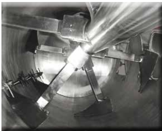
Plow agitator with X-mas tree style choppers
