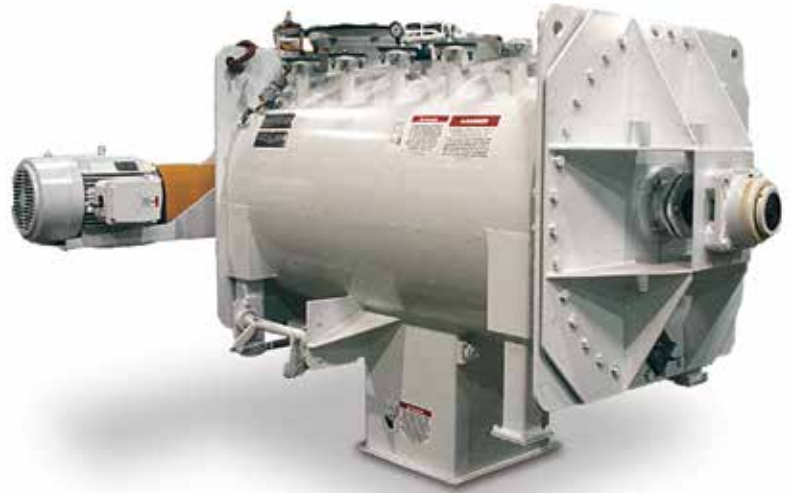
45 ft 3 reactor with jacketed mixing vessel, Kynar ® coated carbon steel and Hastalloy components (corrosive rubber reclamation).
