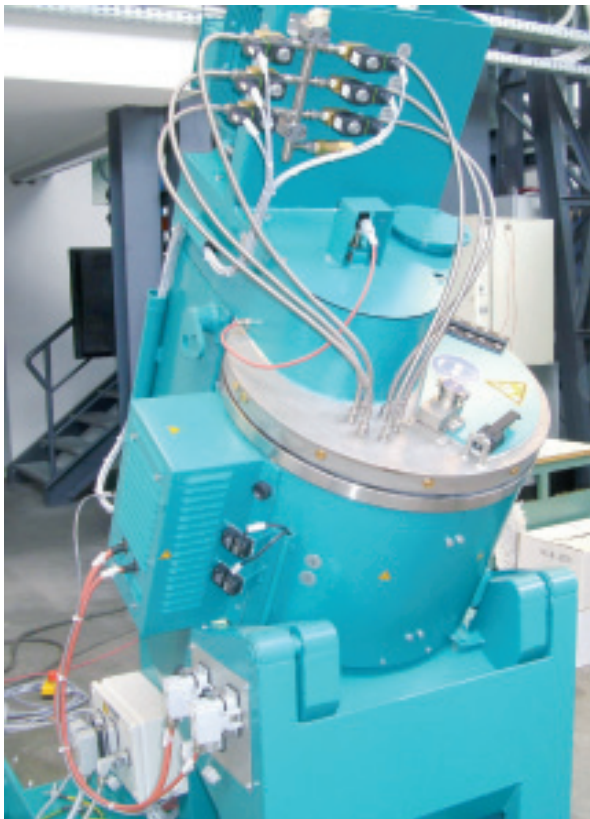
Fig. 4 ROST mixer for plasticizing and granulating paraffin-containing mixes with quartz lamp heaters and CO 2 liquid gas cooling
