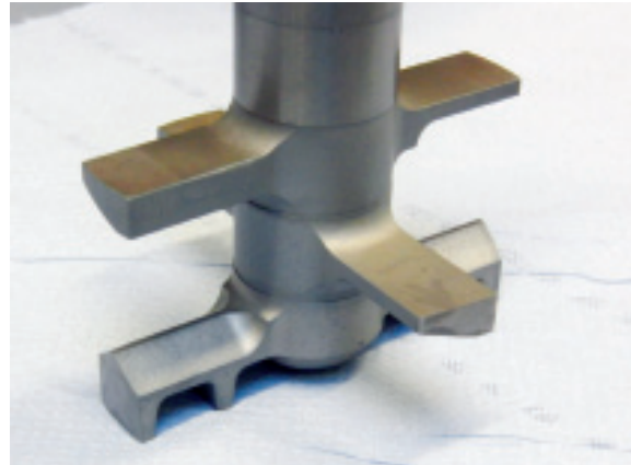
Fig. 3 Mixer with solid carbide studded-type rotor and pan lining made of polyurethane (left) – solid carbide star-type whirler (right)
