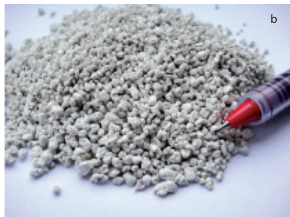
Fig. 8 Plasticized, comminuted and subsequently granulated feedstock based on different binder systems (a and b)
