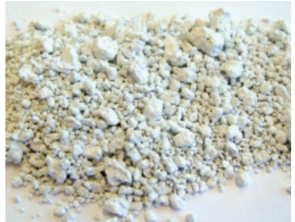
Fig. 7 Granulates produced by comminution of the plastic compound with simultaneous cooling
