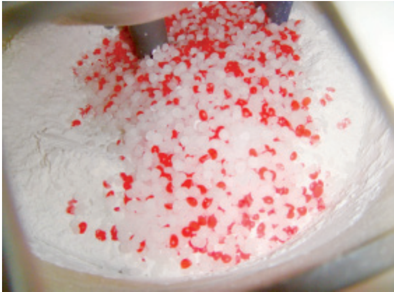
Fig. 2 Receiver for the mix of dry materials and thermoplastic
