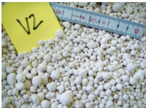
Fig. 8 Plasticized, comminuted and subsequently granulated feedstock based on different binder systems (a and b)
