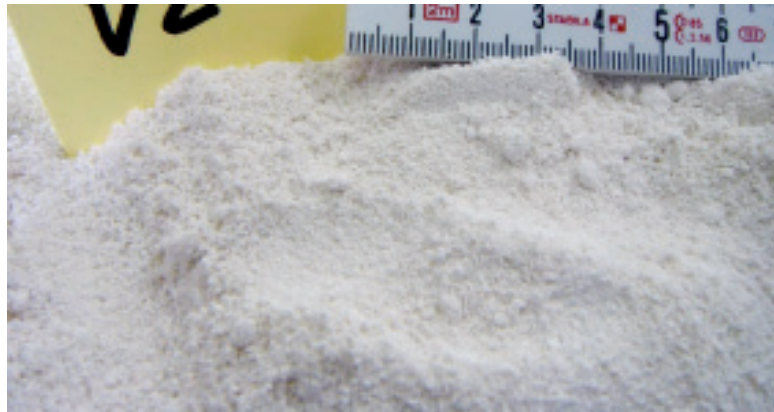
Fig. 10 Fine-grained granulate structure obtained by melting the raw materials mix without plastic phase
