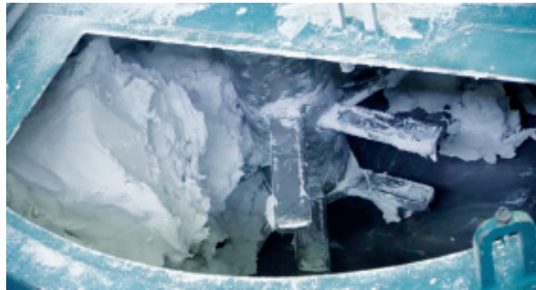
Fig. 1 View into a 150 l EIRICH mixer in the process of preparing high-plasticity ceramic bodies for extrusion
