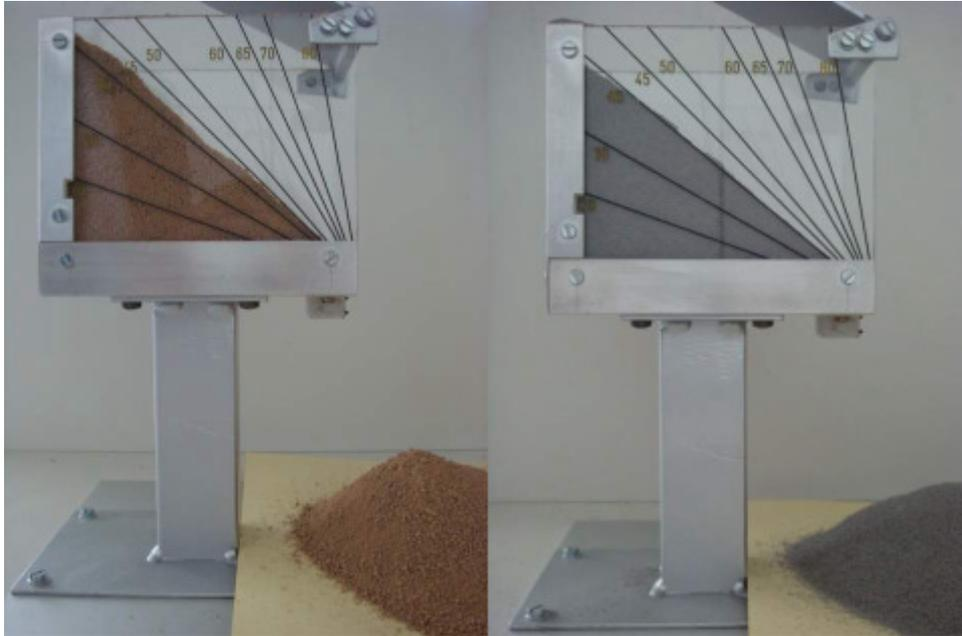
Figure 5: flowability of dry granules      Figure 6: flowability of spray granules
