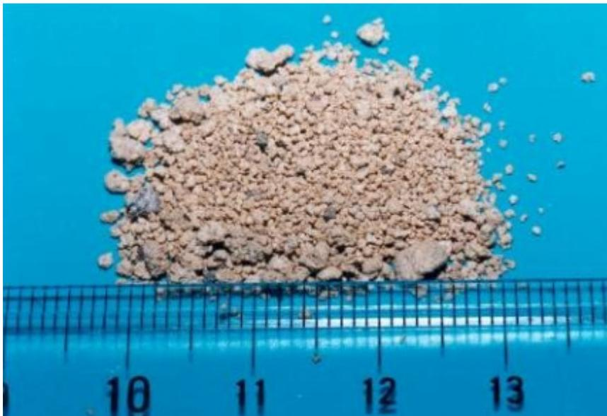
Figure 2: granules after discharging from the mixing granulator
