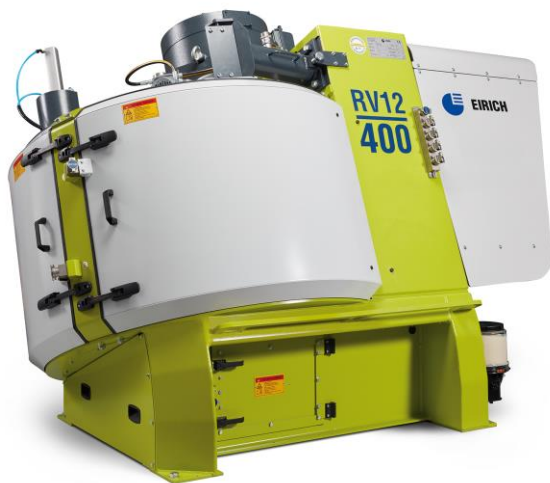
Fig 1: EIRICH Intensive Mixer Type RV12 with a capacity of 400 liters
