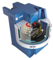
Unlike conventional mixing systems like planetary mixers, the MixSolver® features a rotating mixing pan with an eccentrically arranged mixing tool. This creates perfectly dispersed slurries in 15-20 minutes, with low energy consumption.
