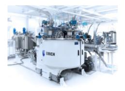
Downstream from electrode slurry processing in the MixSolver<sup>®</sup>, EIRICH's ContiFeeder<sup>®</sup> process ensures a continuous feed of high-quality electrode mix.
