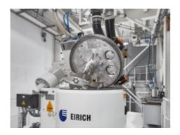
The MixSolver<sup>®</sup>, shown here with the eccentrically arranged mixing tool, is optionally available with EvacMix<sup>®</sup> for directly degasified slurries, a double jacket for a temperature-controlled process, and explosion protection.
