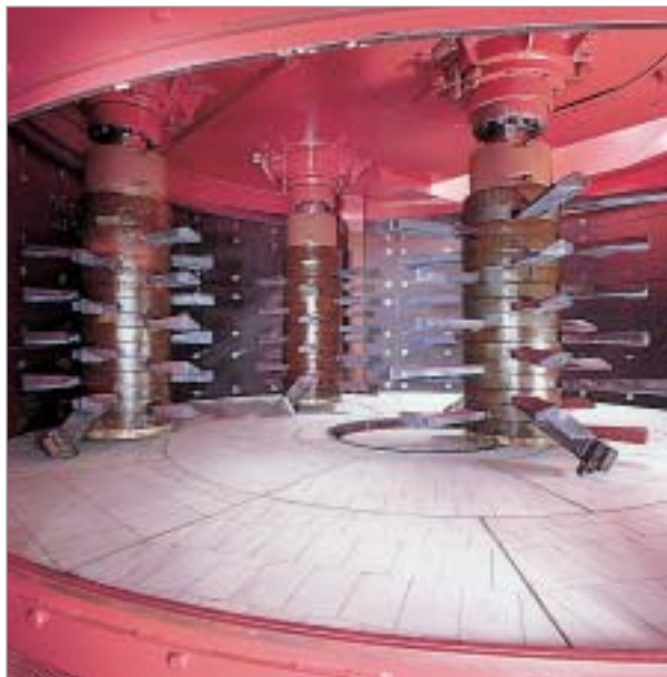
Figure 25: Continuously working mixer for iron ore, 6000 litres of useable volume
