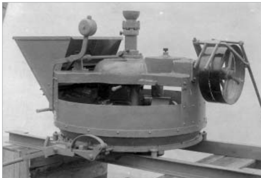
Figure 8: Planetary mixer, around 1910
