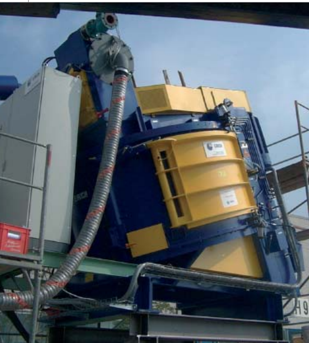
Figure 24: Eirich vacuum mixer, type RV 23 Vac
