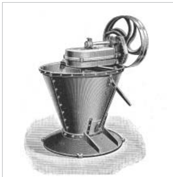
Figure 6: Funnel shaped mixing machine, around 1908 [19]
