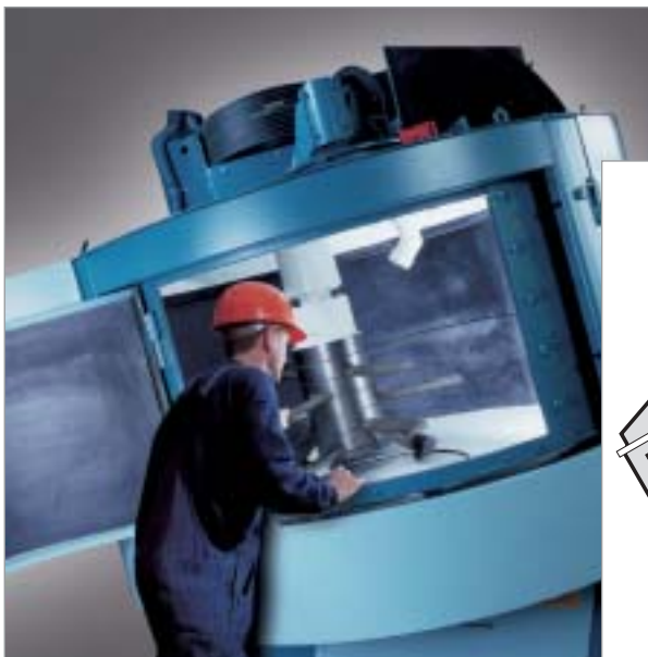
Figure 14: Eirich mixer with an inclined mixing container
