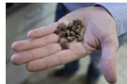
This is the shape of the new blended fuel granules from waste plastic and biomass
