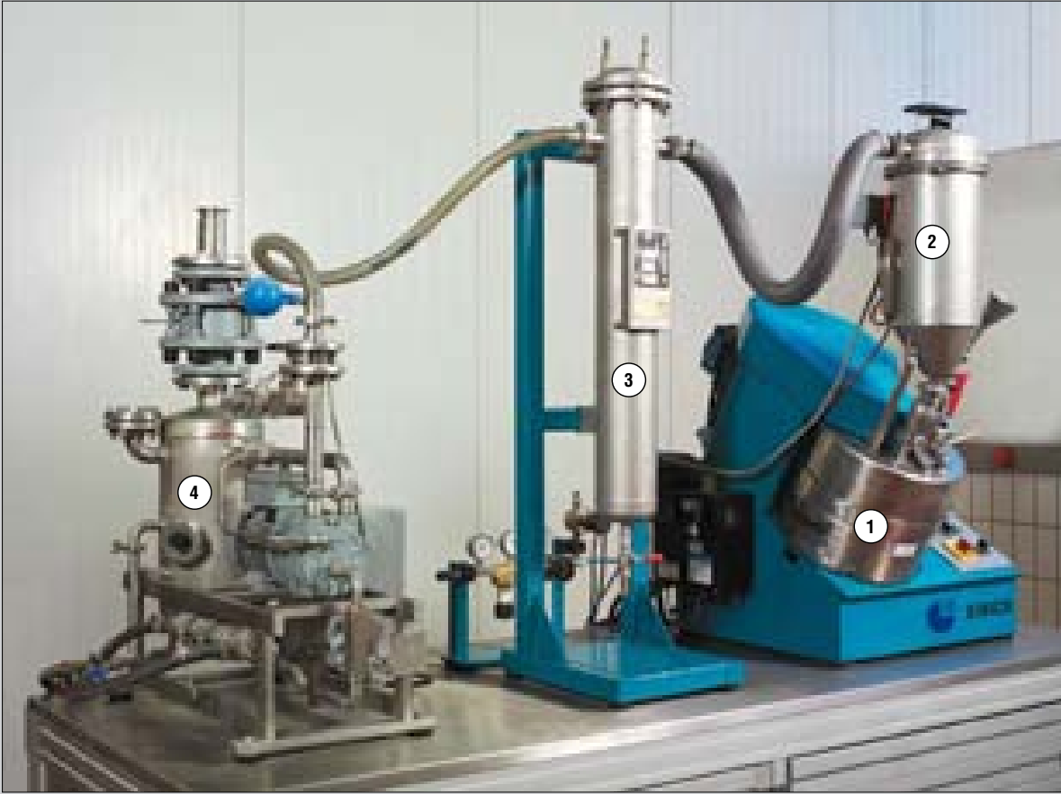
Fig. 5.1: R02VAC EVACTHERM® explosion-proof mini plant with mixing reactor (1), top-mounted vapor filter (2), condenser with integrated liquid collecting container (3) and vacuum pump module with pressure controller (4).
