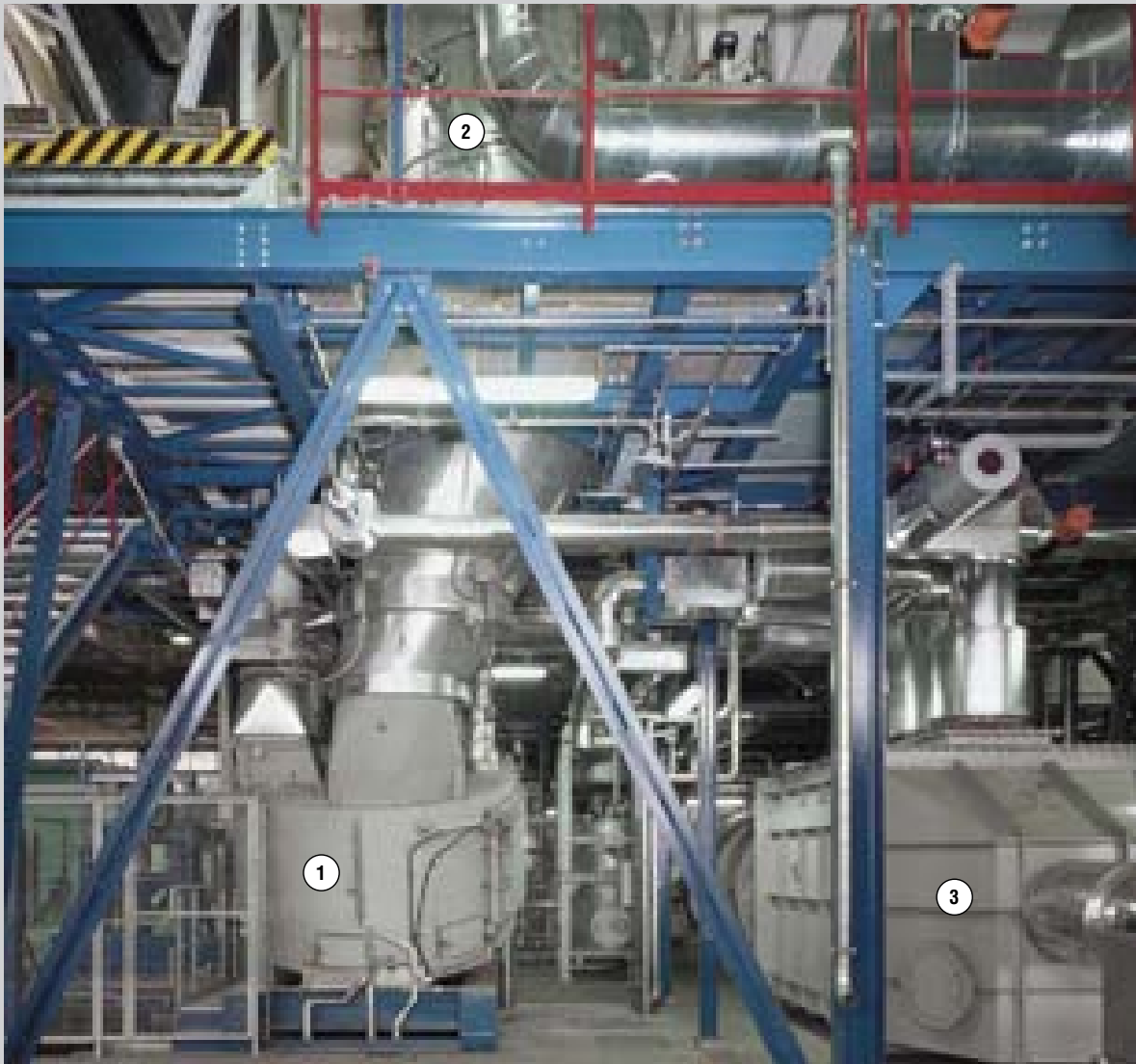
Fig. 11.1: Drying system for the treatment of industrial sludges: Drying capacity of 1000 kg/h, with an EVACTHERM® intensive mixer RV23VAC (1) vapor filter (2) steam superheater (3)
