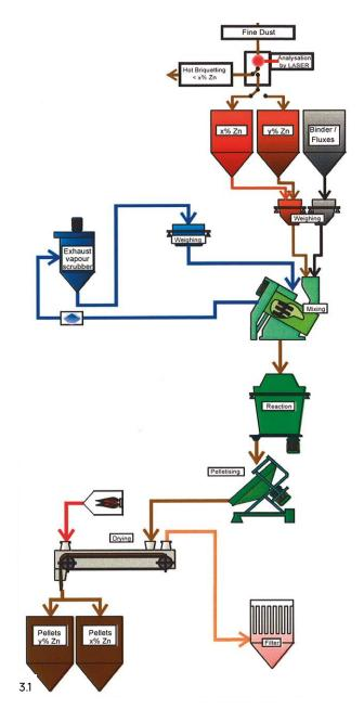
Fig. 3.1: Pelletising system for BOF dusts
