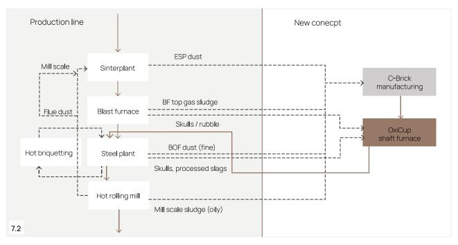
Fig. 7.2: Material recycling with the OxyCup process
