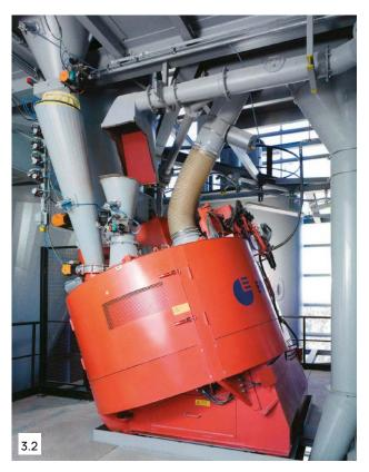
Fig. 3.2 Eirich mixer 1,500l batch volume
