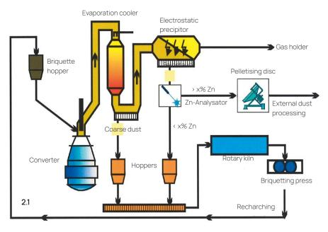
Fig. 2.1: Recycling of residual BOF dusts at Voest Alpine Stahl in Linz, Austria
