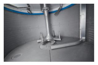
Mixer interior with pin-type rotor, cleaning nozzles, humidity probe
