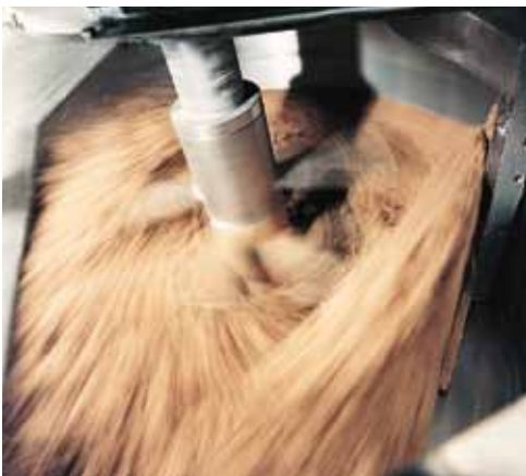
Material stream in the EIRICH intensive mixer
