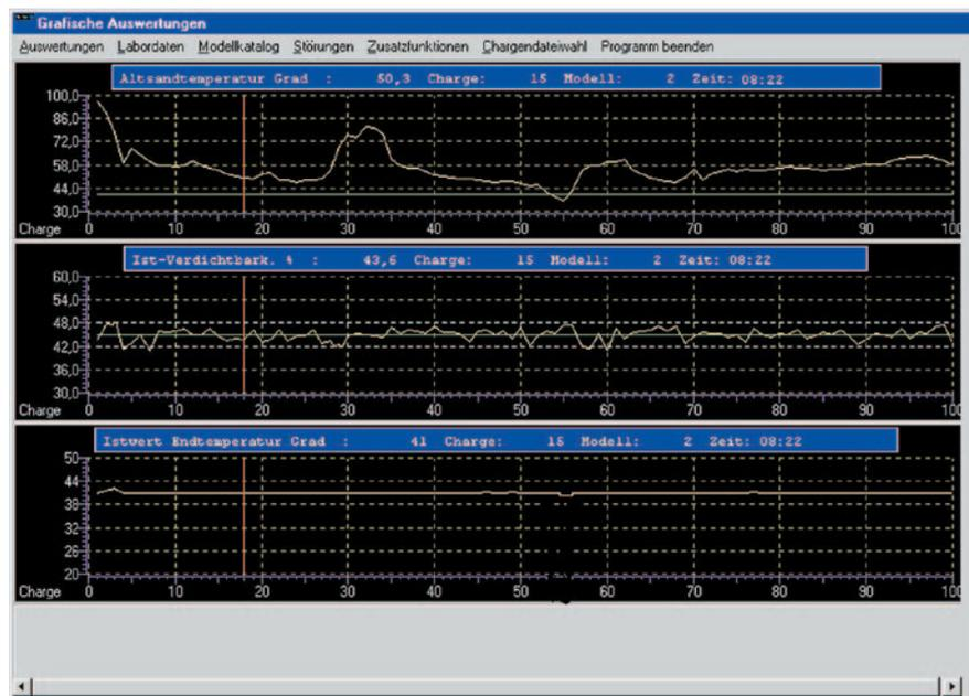
Fig. 8: SandExpert: View of the temperature curve of the return sand and the newly prepared molding material
