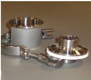
Tri-clamped ferruls for liquid additoin port
