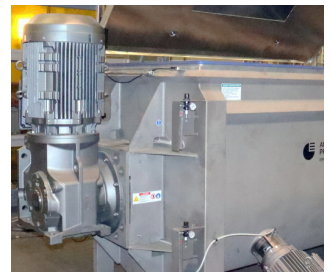
Direct drive, right angle shaft mount
