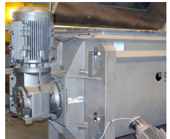
Direct drive, right angle shaft mount
