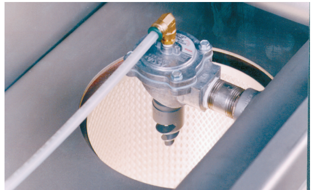
Pulse jet air divertors insure efficient cartridge cleaning. Timers control both frequency and duration of air blast.
