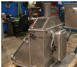
NEMA 9/XP dust electricals
