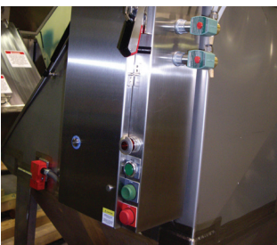
NEMA 4X-SS water tight combination pulse jet timer, FVNR starter and disconnect
