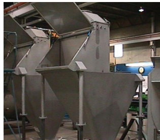
FBD with surge hopper extended to accomodate customer's bulk bag discharge frame
