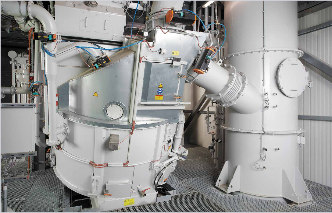
Fig. 1: Evactherm-Mixer, cooling – preparation – mixing in one aggregate.
