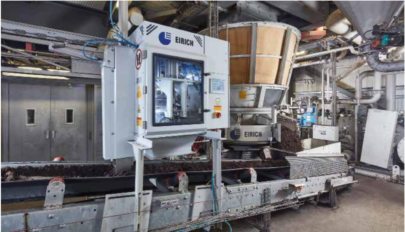
Fig. 3: Eirich inline tester QualiMaster AT1, the heart of the quality assurance in molding material preparation
