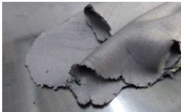
Dry electrode film made from structured electrode mixture prepared in the Eirich mixer
