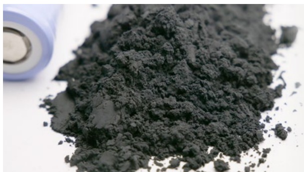
Structured electrode mixture produced in the Eirich mixer.
