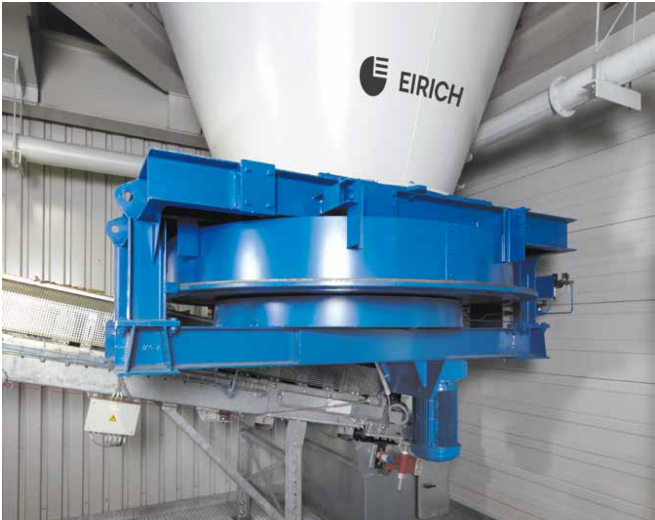
UE24 table feeder Silo discharge unit version
