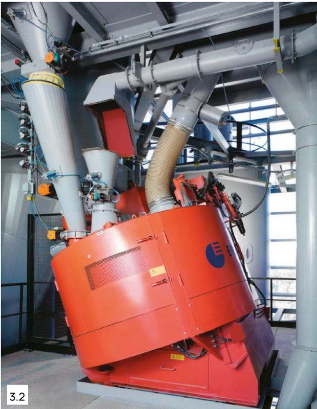
Fig. 3.2 Eirich mixer 1,500l batch volume
