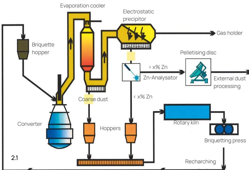
Fig. 2.1: Recycling of residual BOF dusts at Voest Alpine Stahl in Linz, Austria
