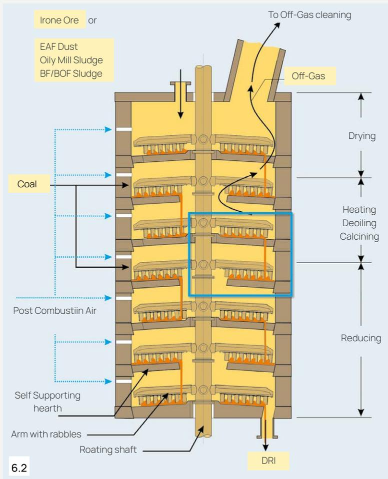
Fig. 6.2: Functioning principle of a multiple hearth furnace
