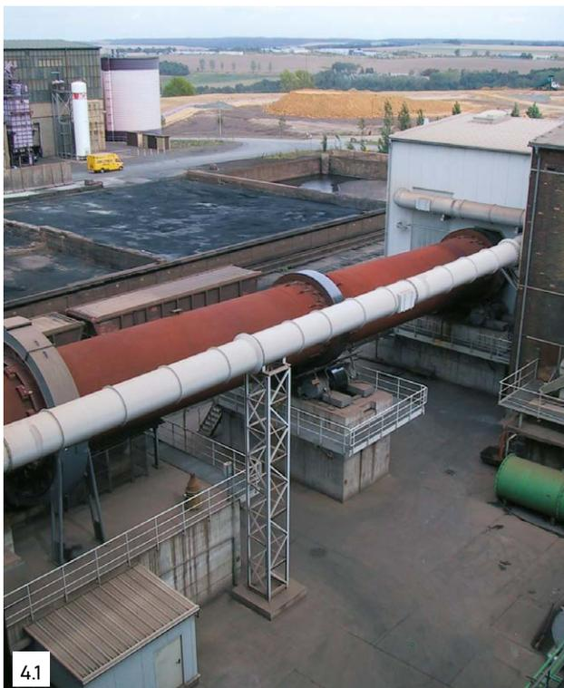
Fig. 4.1: Waelz kiln 2 at BUS Zinkrecycling in Freiberg, Germany
