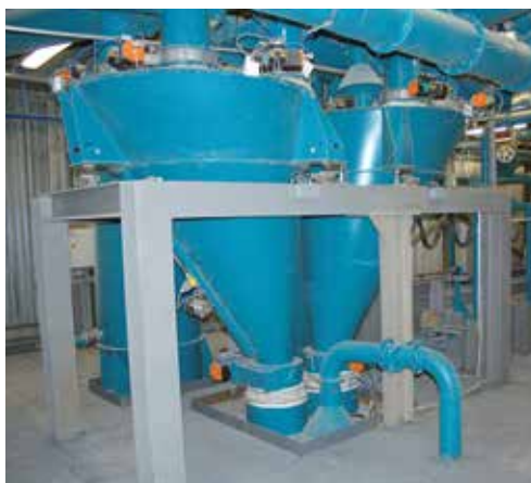
Sand and binding agent scale
