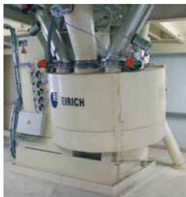
Eirich intensive mixer RV19 with a 10° tilt
