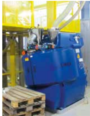
Eirich Intensive mixer R12W
