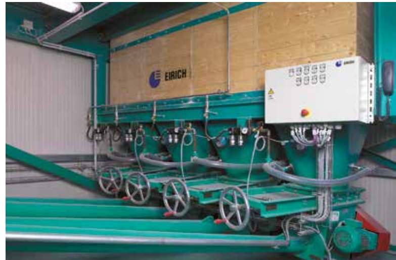
Additive storage and feeding
