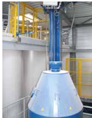
Lift- and swivel hoist
