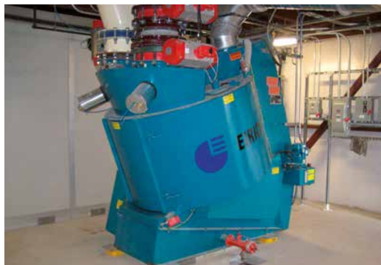
Eirich intensive mixer RV15 with a 10° tilt
