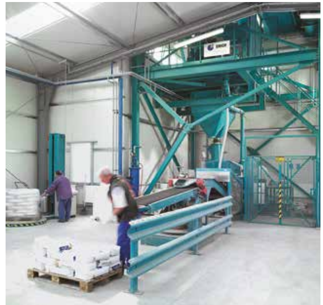
Single-spout packer with manual palletizer
