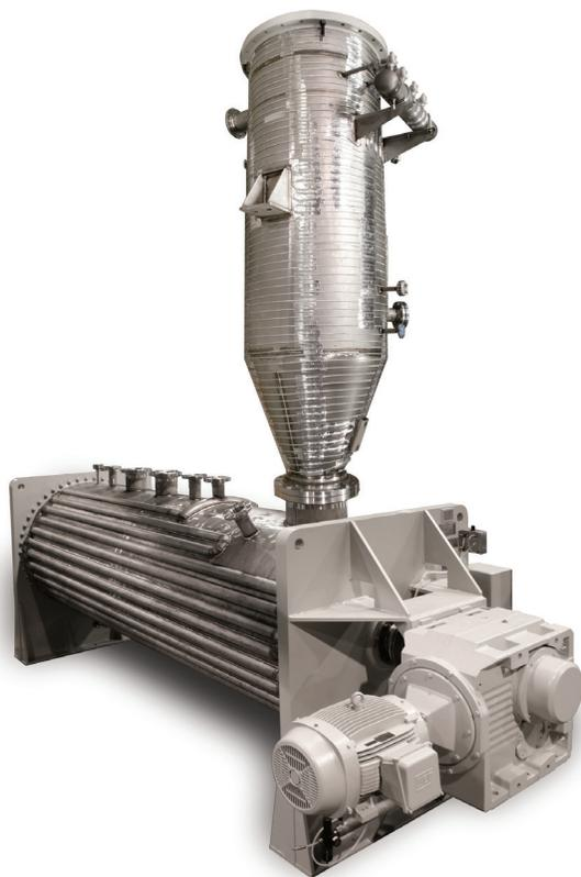
200 ft<sup>3</sup> vacuum dryer/reactor with half-pipe jacketed mixing vessel, 2205 duplex stainless steel and electrically heated dust collector.
