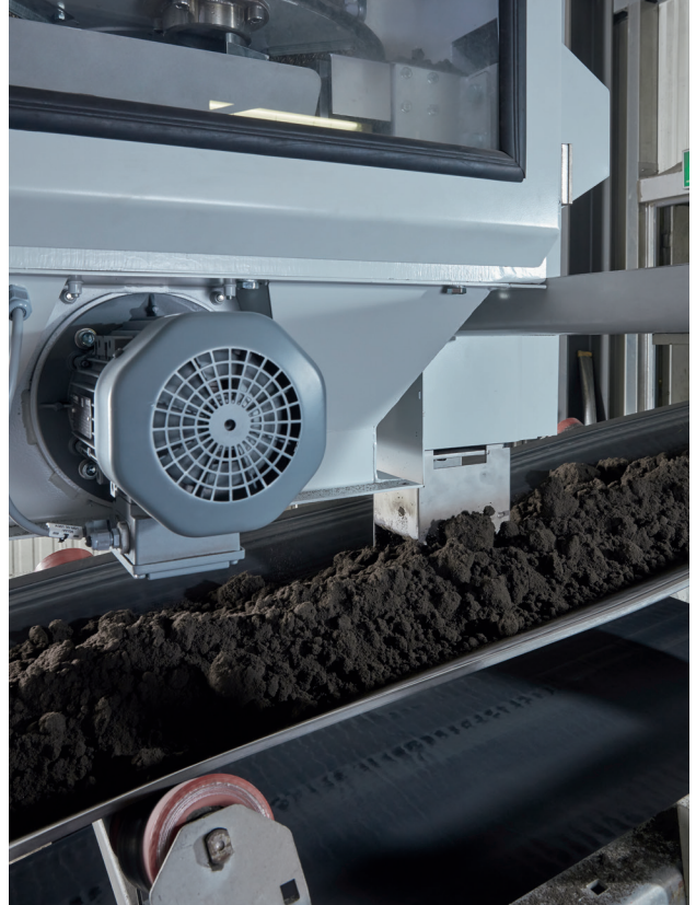
The inline test device QualiMaster AT1 removes samples immediately downstream of the mixer from above the conveyor. As an option, a sample crusher can be incorporated in the basic version AT1 Eco.
