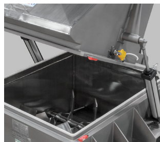
Dual pneumatic cylinders for opening cover
